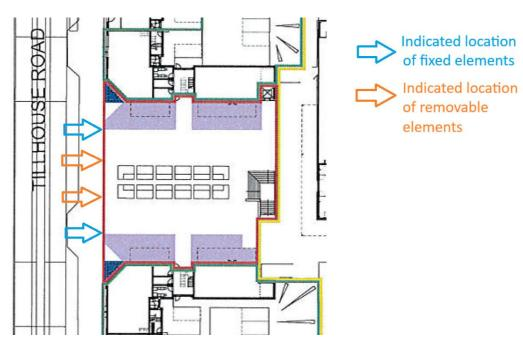
In order to prevent vehicular traffic, it is suggested that elements should be spaced 1.5m apart, resulting in the need for 16 elements in total.
